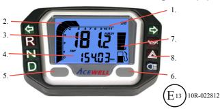
Thanks for purchsaing an Acewell ATV/Motorcycle/Scooter computer. This manual is specifically designed for ACE-3XXX series. The ACE-3100/3150 does not have any extra LED indicator. The ACE-37XX/38XX series has 4-8 LED indicators. Different models have different LED indicators; a fuel meter is optional, but all other functions are the same. You may find that the photo has a set of LED indicators different from your computer; the photo is for reference
